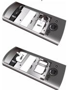
As shown, align the metallic connectors on the battery and battery slot. Insert the battery until it is locked.
